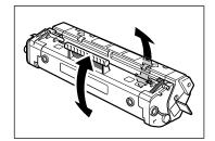
Place the cartridge on a sturdy surface. Snap the tab at the end of the cartridge backwards and fold it back and forth until it is loose. Then pull the sealing tape in the direction indicated in the illustration below.
