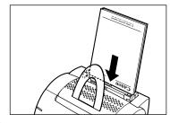
Adjust the paper guides according to the size of the paper loaded. Be sure to adjust the paper guides so that there is no space between each paper guide and the edge of the stack of paper.
