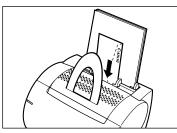
**2** Adjust the paper guides according to the size of the paper loaded.
